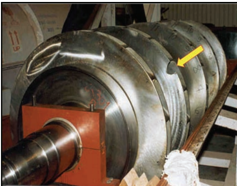
Figure 1. Failure in centrifugal compressor initiating in fabrication weld.
