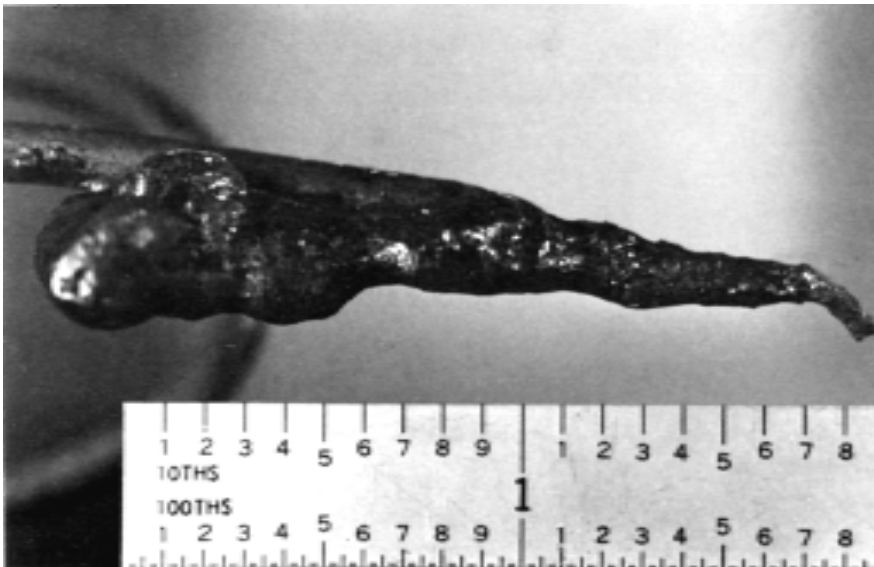
Copper wire damaged due to melting not arcing
