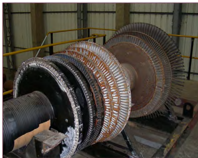
Figure 1. After only a short period of operation, the turbine became contaminated with deposits.
