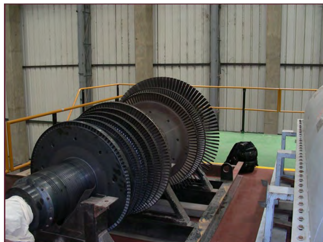
Figure 2. The mill improved operating practices and chemical monitoring that made a tremendous improvement in the turbine’s appearance.
