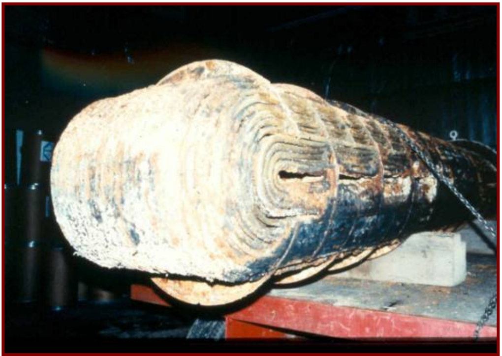
Figure 1. Severely scaled floating head tube bundle (cooling water on shell side).
