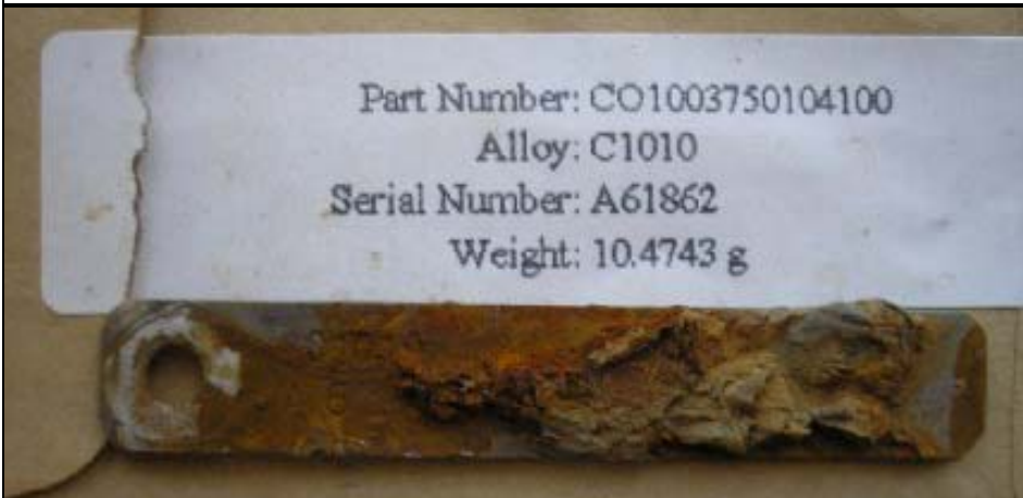
Figure 3B. Side of Corrosion Coupon with Heavy Corrosion.
